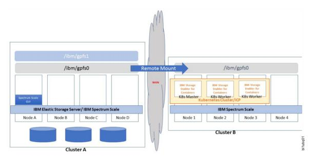
Figure 9. Sample configuration supported by IBM Storage Enabler for Containers
