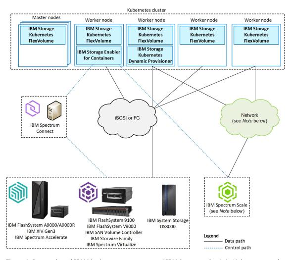
Figure 1. Integration of IBM block storage systems and IBM Spectrum Scale in Kubernetes environment
